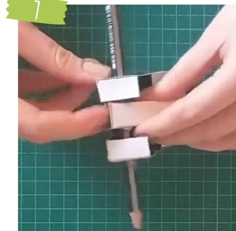
Run a pencil through the holes of part 1 and 2 as shown to join them. Tape the pencil to part 2 so that it is unable to rotate.
